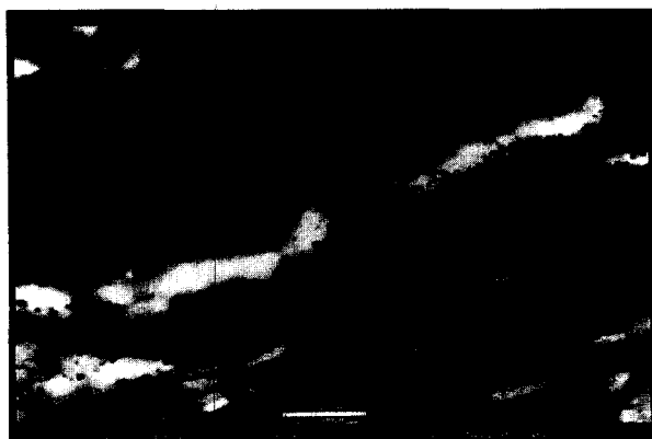
Fig. 8. Environmental scanning electron micrographs of the surface of the copolymer matrix after bioadhesion to duodenal mucosa.
